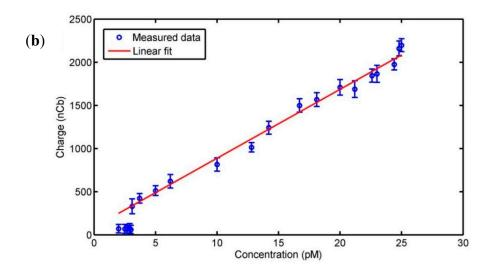
In the horizontal range of the first five points in Figure 3b, the increase of dopamine concentration did not lead to an increase in signal. Thus, 3.1 pM was the lowest detected dopamine concentration with the membrane sensor presented in this study.
