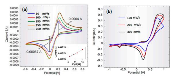
It is seen that the numeric ratio between the current peaks is almost unity (example in figure: 0.0004 A/0.00037 A) and that the peak potentials are independent of the sweep rate. The inset in Figure 2a
