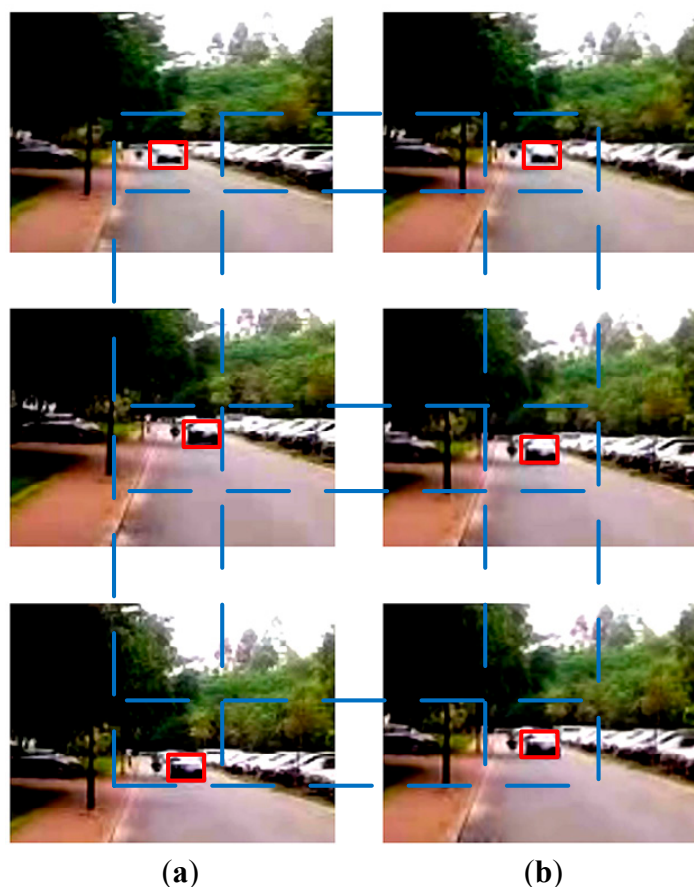
Figure 8. (a) the vibrating images; (b) those compensated by the optical stabilization method, using two DMs, the car in the image sequences was marked in red line.
