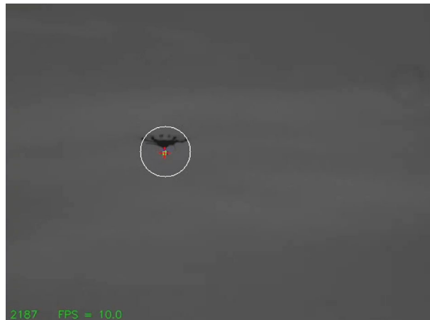
Figure 4. Image from the machine vision tracking camera. The red cross shows the detected position of the beacon LEDs. The white circle shows the tip/tilt mirror actuation range, centred on the predetermined hotspot.
