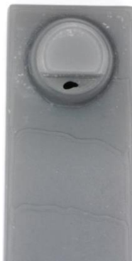
Figure 6. Printing defect observed in all 0^\circ samples at the same position on the build platform.
