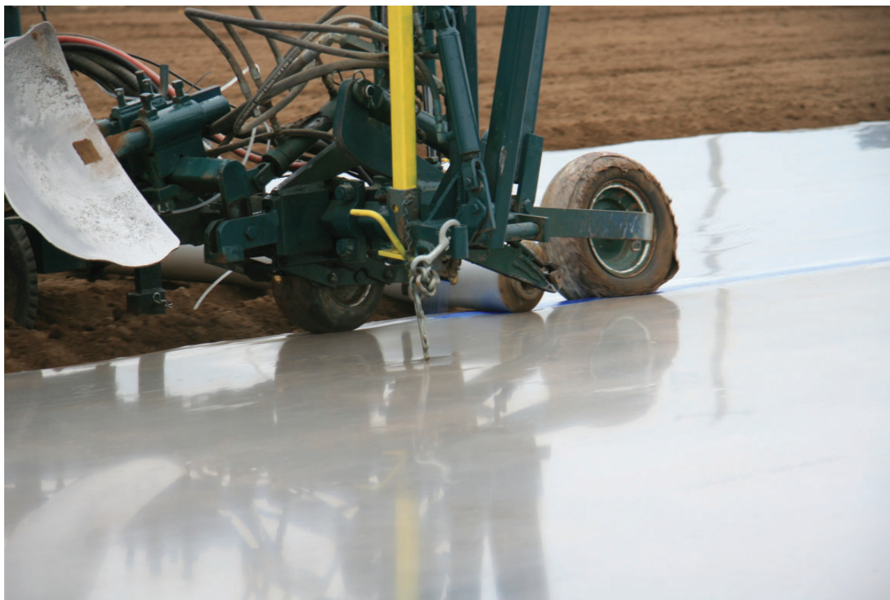
Fig. 4. Use of totally impermeable film and gluing overlapping tarp edges during soil fumigation.
