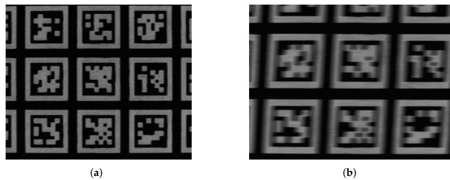
Figure 6. Camera image of moving objects captured (a) with a global and (b) a rolling shutter.
