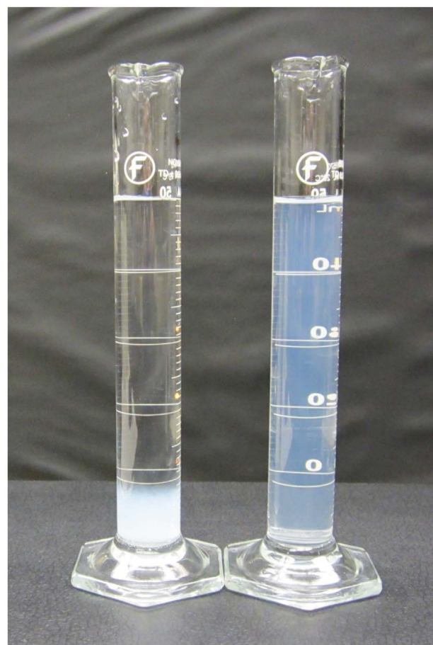
Figure 2 | Freshly prepared apatite nanoparticle suspensions in the absence of CMC (left) and in the presence of CMC (right).
