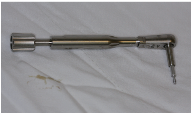
Fig. 1. Ostell SmartPeg was connected with 5 Ncm using hand torque wrench.
