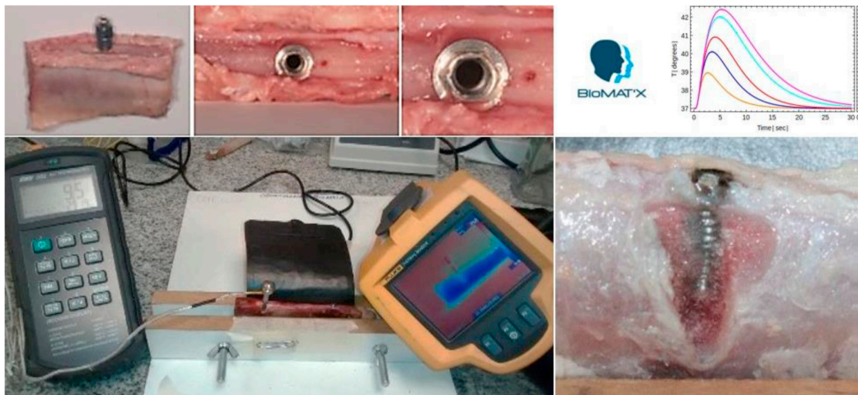
Figure 8. Experimental Set-up; developed in-House (at the BioMAT'X R&D&I Laboratory—Haidar Lab, CiiB, Faculties of Medicine and Dentistry, Universidad de los Andes, Santiago de Chile) as an ex-vivo heat distribution model employing human patient-grade titanium dental implants placed into porcine ribs (without coolant) and thermal changes monitored/recorded (quantified) using a CorDEX TP3R ToughPix DigiTherm Digital Thermal Camera ( an ongoing investigation ).
