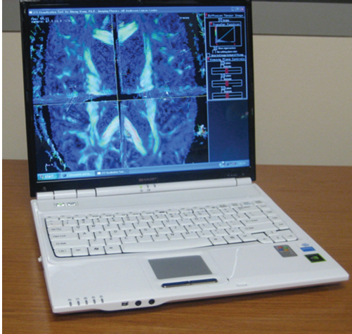
FIGURE 3: Photograph of the stereoscopic DTI processing and visualization tool. The laptop is equipped with a glasses-free LCD monitor. The laptop computer can operate in stereo or nonstereoscopic mode: the user can switch between modes by pushing a button. In stereoscopic mode, the LCD operates in 512 \times 768 matrix size, and while in nonstereoscopic mode the LCD operates at 1024 \times 768 .
