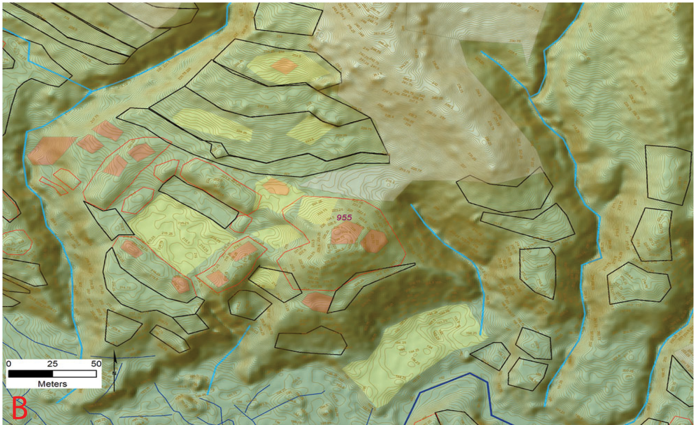
Fig 17. Eastern 'cache' location (B) at site 955 ( la Ciudad del Jaguar ) within the Valle de la Fortaleza (T1). Location of section at the site and a legend are shown in Fig 6. Digitized features are shown over a composite hillshade view taken from 16 different angles draped on a color shaded DSM with a resolution of 1 m/pixel. Contour interval is 25 cm. All visualizations created using high resolution aerial LiDAR.
