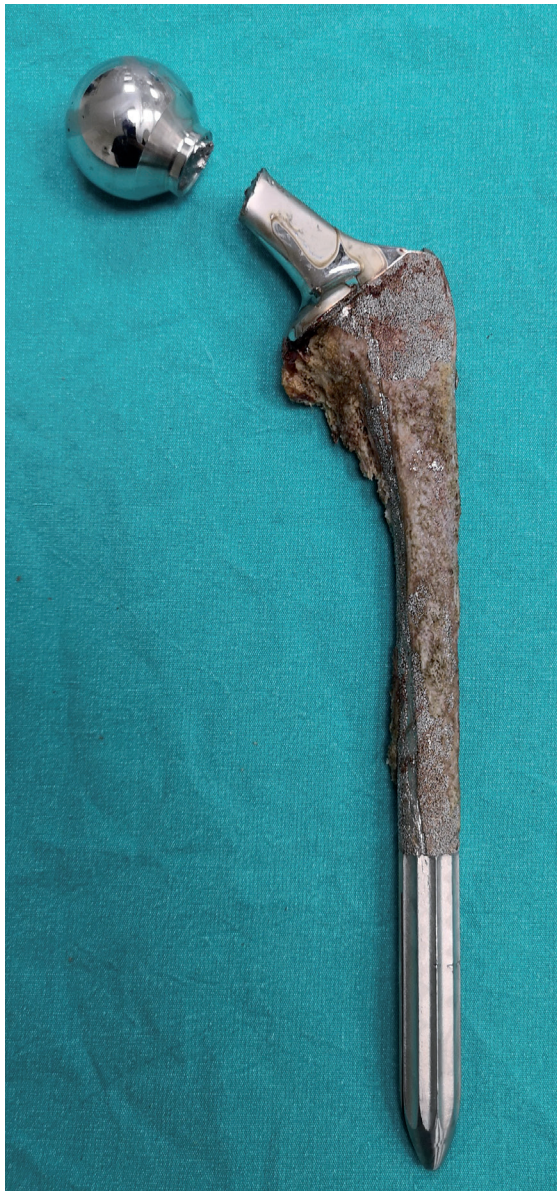
Figure 2. Trunnion fracture of the femoral stem.
