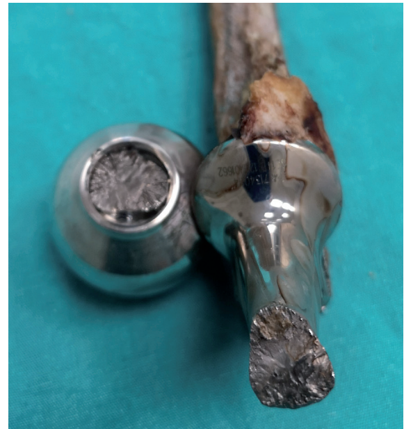
Figure 3. The femoral stem and the trunnion fracture surface.
