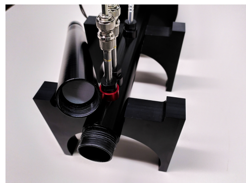
(b) Impedance tube AED 1000 with specimen and 1/4" microphones
