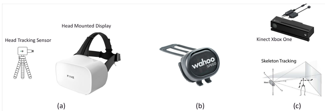
Figure 2. Sensors used in the development of the Cycling and Hazard Perception VR simulator. (a) FOVE VR Headset, (b) Wahoo RPM Cycling Speed Controller, and (c) Microsoft Kinect.
