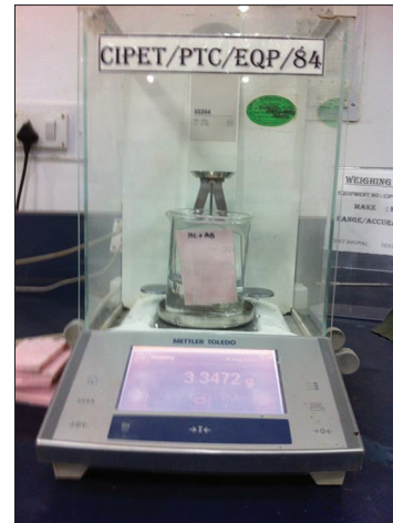
Figure 6: Weighing of specimen in water on an analytical balance
