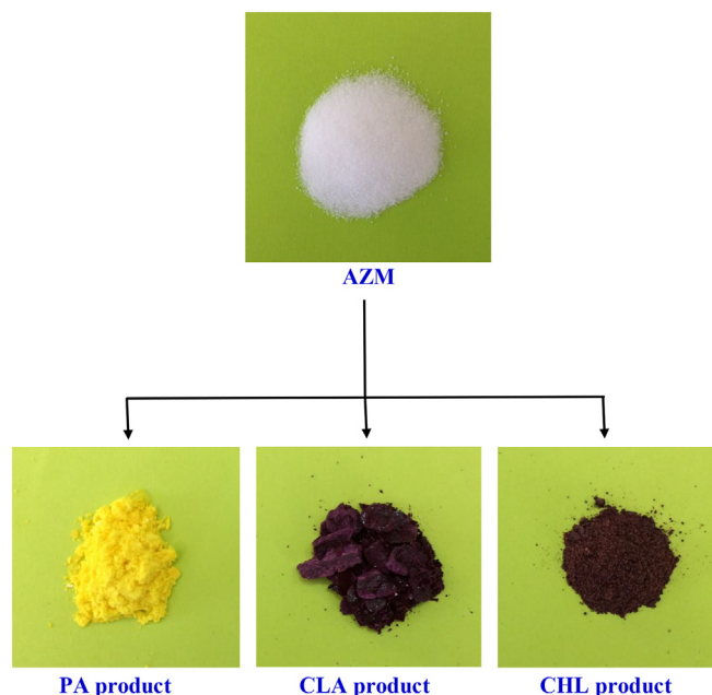
Fig. 2. Free AZM (white) and its solid CT products: AZM-PA complex (canary yellow), AZM-CLA complex (violet), and AZM-CHL complex (brownish-red).
