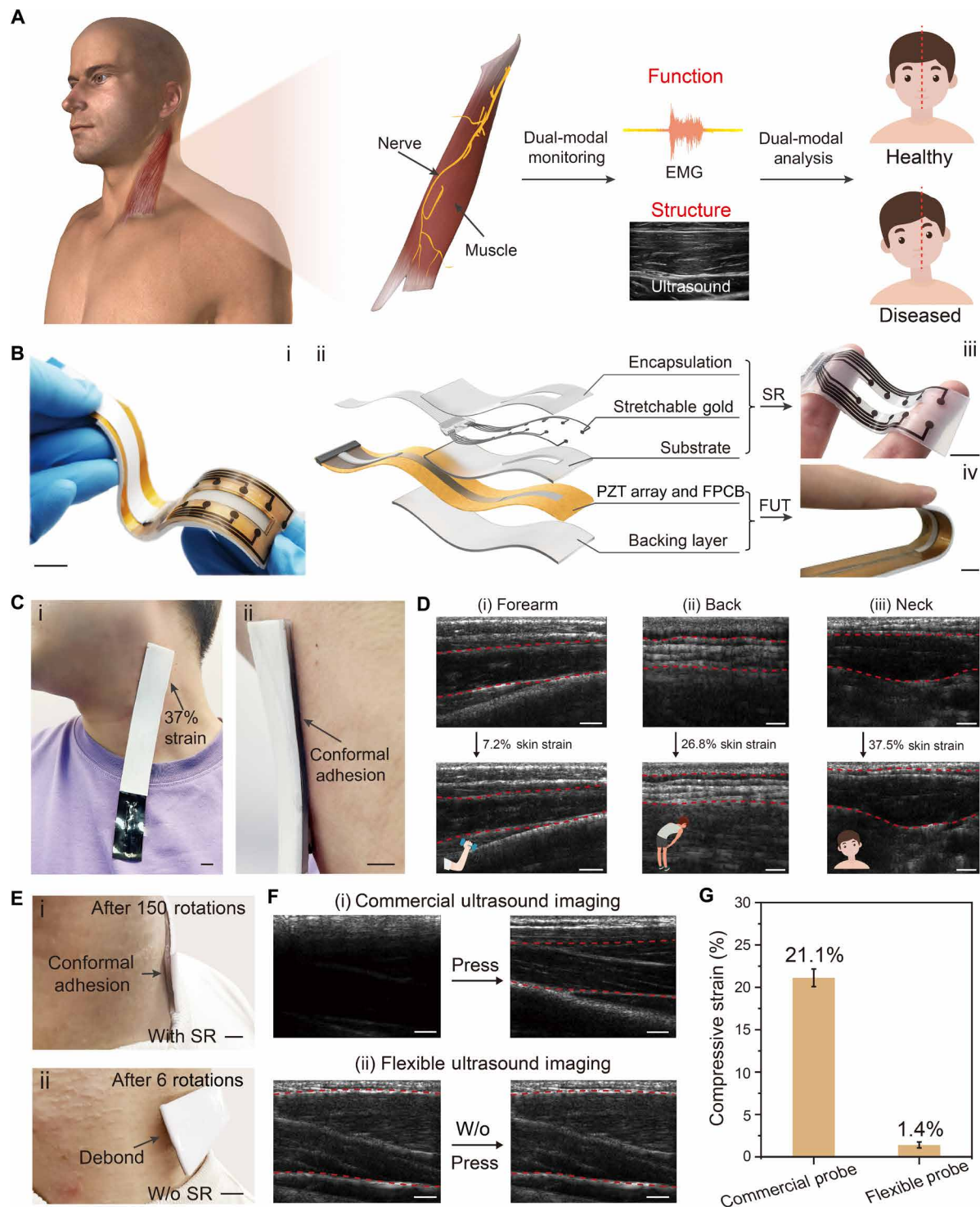
Fig. 1. Overview of the wearable integrated structural-functional sensing patch for in situ synchronous monitoring of muscular ultrasound imaging and functional signals. (A) Pictures to demonstrate one of the targeted muscles: SCM muscles that can deform largely with mechanical strain of ~30% in skin. The structural-functional sensing will benefit the precise diagnoses, e.g., muscle fibrosis and disorders. (B) Images of the integrated (i) and layered (ii) WSFP, as well as images of separate the SR layer (iii) and the FUT (iv). Scale bars, 1 cm. (C) Images depicting the conformable attachment of WSFP on neck. Scale bars, 1 cm. (D) Ultrasound imaging of the brachioradialis, erector spinae, and SCM muscles was performed at multiple instances when the skin surface strain of the forearm, back, and neck monitored by WSFP reached 7.2, 26.8, and 37.5%, respectively. Scale bars, 5 mm. (E) Attachment states of the FUT with a 2-mm SR layer after 150 rotations of the neck (i) and without a SR layer after 6 rotations of the neck (ii). Scale bars, 1 cm. (F) Commercial rigid ultrasound probe is used for muscle structural imaging, and pressure is required causing structure change to the muscle (i), which indicates that the commercial ultrasound probe could not reflect the real structure of the muscle, and FUT is used for muscle structural imaging without pressure required and muscle thickness appears notably larger than that captured by the commercial probe (ii). Scale bars, 5 mm. (G) Commercial ultrasound probes cause 21.1% tissue deformation during compression imaging, whereas flexible ultrasound probes induce only 1.4% tissue deformation when attached directly for imaging.
