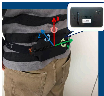
Figure 1. To measure sensor data required for pedestrian dead-reckoning (PDR), we asked the employees to carry the smartphone during the operation.
