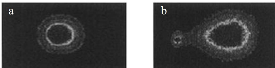
Figure 2. The comet assay images of a healthy cell (a) and a damaged cell (b). The damaged cell is observed as a bright comet head with a dispersive tail.
