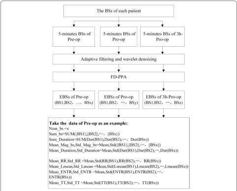
**Fig. 2** Overview of BSs data acquisition, processing, and analysis. BS is short for the bowel sound. Pre-op is short for before operation. Pro-op is short for after operation. 3 h-Pro-op is short for 3 h after operation. FD-PPA is short for FD-peak peeling algorithm. EBS is short for the effective bowel sound
