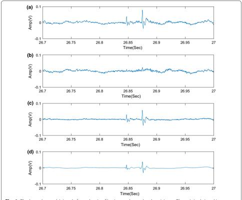
**Fig. 1** The bowel sounds' signal after adaptive filtering and wavelet denoising. **a** The original signal is obtained from the microphone after amplification without any cancelation, and **b** the ambient noise is collected from the other microphone. **c** The signal after LMS adaptive filter. **d** The signal after wavelet denoising
