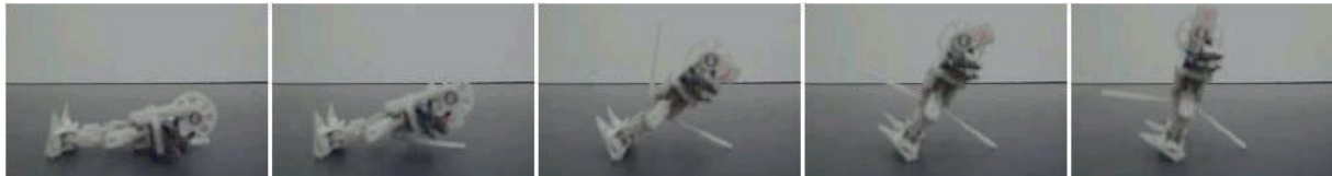
FIGURE 32: Self-righting process of a jumping robot designed by Zhao et al. [99].
