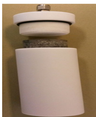
Figure 4. A schematic of the NMR core holder.
