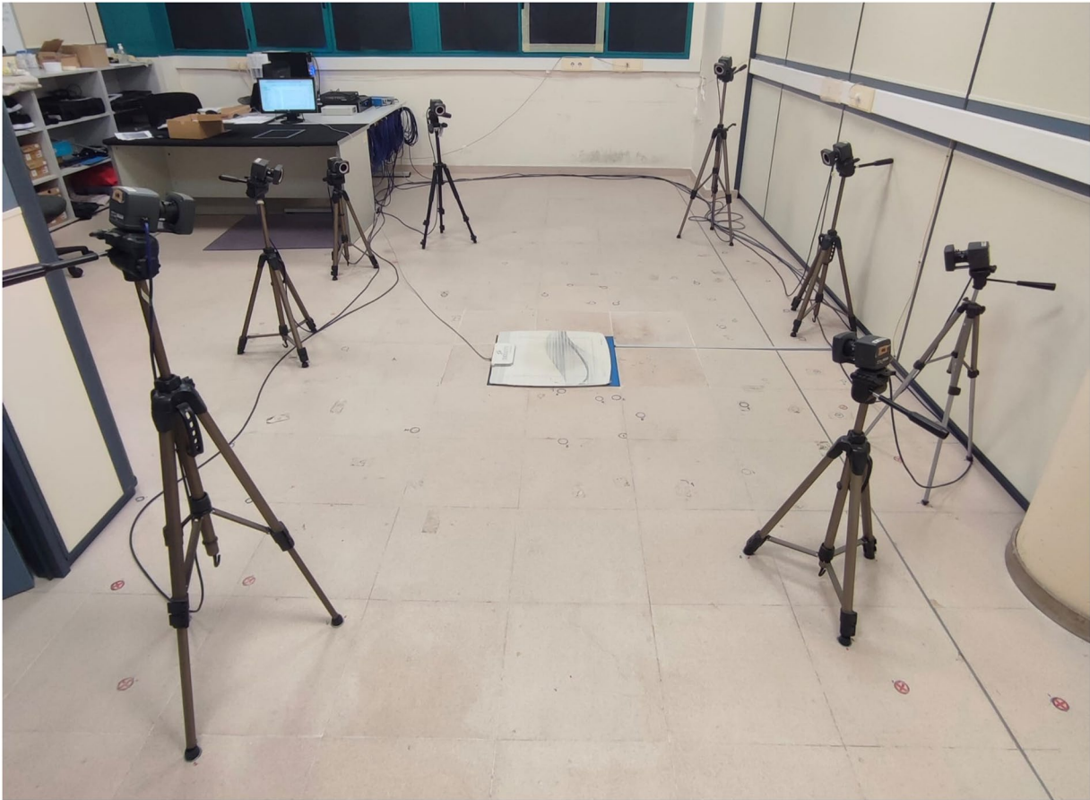
Fig. 2 View of the distribution of the 8 Vicon cameras and the location of the pressure platform in the middle of the walkway.
