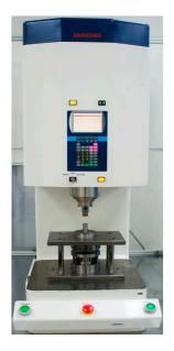
Figure 8. The electro press for the micro-channel array forming process (JANOME JP-5004).
