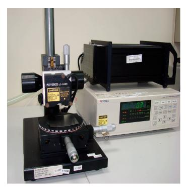
**Figure 9.** Laser displacement system (Keyence LC-2430) for contour measurements of stamped stainless steel plates.
