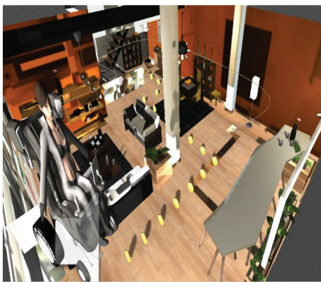
FIGURE 7: The training trajectory is divided into three parts: driving in a straight line, right turn, and left turn.
