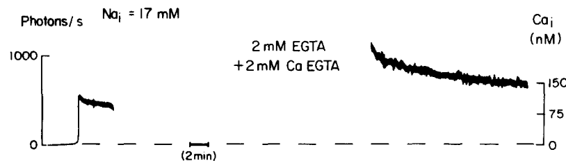
FIGURE 1. The effect on resting glow of equilibrating an axon with EGTA buffer containing \sim 4 mM total chelator. The axon was initially injected with aequorin and phenol red (220 mM K-salt) and it had a diameter of 0.600 mm. The membrane potential was -60 mV. The external solution was Na seawater with 10 mM Ca. The light trace collection was interrupted during the injection of the Ca buffer, but not so the time base in the record.
