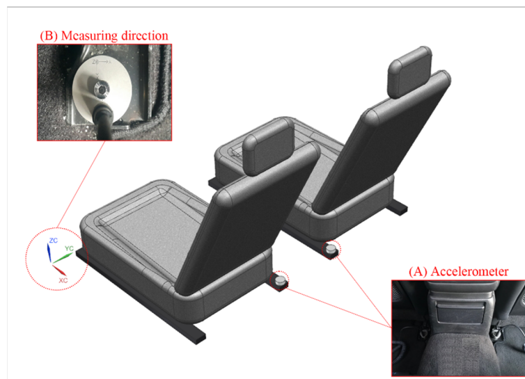
Figure 4. Accelerometer installed to measure the vibration. (A) Accelerometer installed on a seat frame; (B) measurement direction of the accelerometer.
