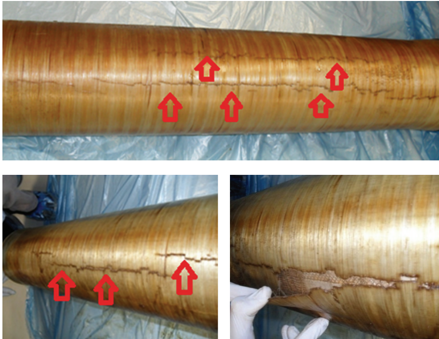
FIGURE 2: Cracked module shells due to high pressure drop (arrows indicate cracks).
