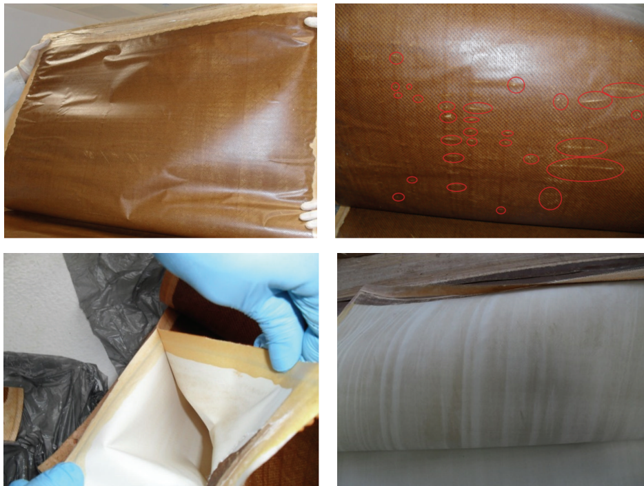
FIGURE 3: Membrane leaves and permeate spacer images taken during physical inspection (circles indicate surface damage).
