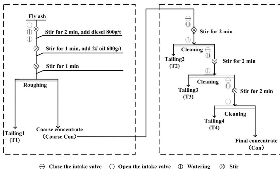
Figure 3. Stage-by-stage release flotation flow diagram.
