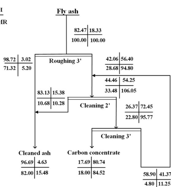
**Figure 8.** Flowchart of quantity and quality for closed-circuit flotation.
