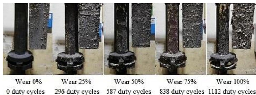
Figure 4. Type B rotor wear.
