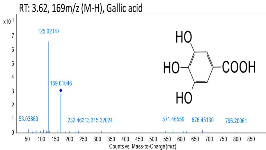
Fig. 2a. The HPLC-MS profile of the bioactive markers gallic acid.
