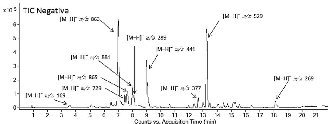
Fig. 2c. The total ion chromatogram of RD1c13 fraction in a negative ion mode.
