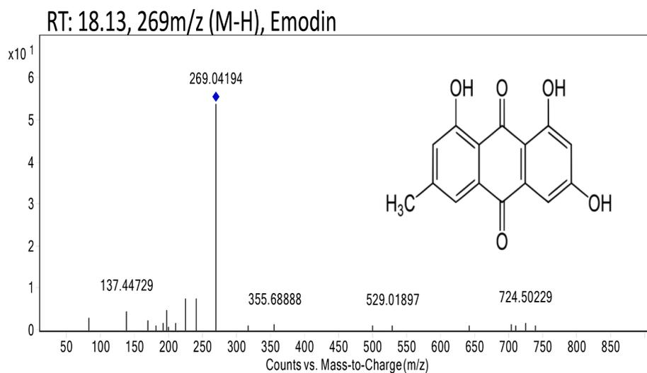
Fig. 2b. Shows the HPLC-MS profile of the bioactive markers emodin.
