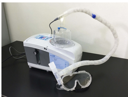
Figure 1 Ultrasonic nebulization system developed in this study.
