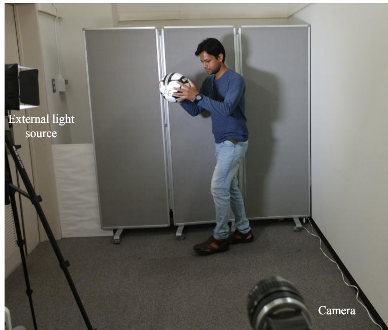
Figure 17. Experiment setup for HFR-projector-camera system using a USB camera as input.
