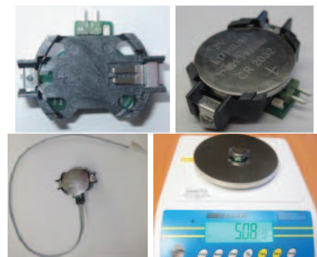
FIGURE 6. Sample of the single piece back mountable micro DBS device.
