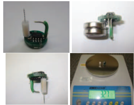
FIGURE 5. Sample of the single piece head mountable micro DBS device.
