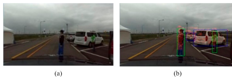
Figure 12. (a) Camera view. (b) Object detection through YOLO and LiDAR point cloud projection on the image plane for object spatial location.
