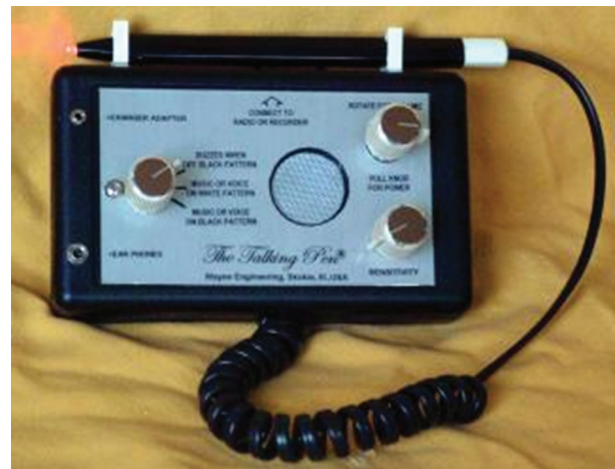
Figure 3. Perceptual-motor pen. Each subject was asked to move a specific pen on the lines of the page. No sound was produced if the pen was moved correctly, while errors in tracing the lines resulted in auditory feedback.
