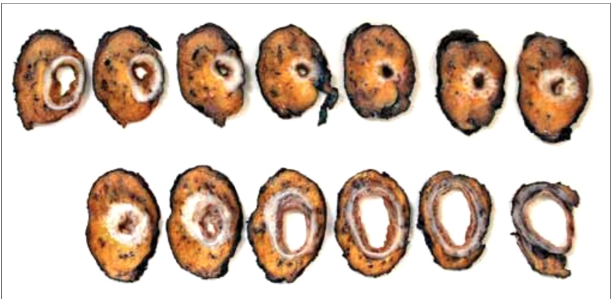
Figure 5. Slice sampling style that covers all circumferential areas, adapted from the method used by Hoorens et al. This figure is taken from the Hoorens et al. study [6].
