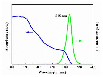
Figure 2. Optical absorption (blue line) and PL (green line) spectra of CsPbBr<sub>3</sub> QDs.
