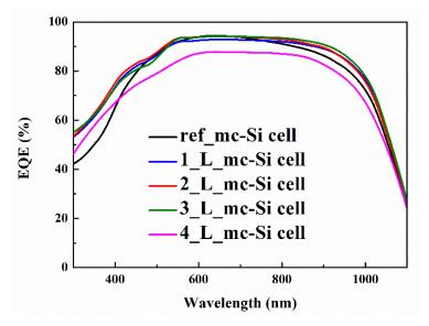
**Figure 5.** External quantum efficiency (EQE) spectra of mc-Si solar cells inclusive and exclusive of CsPbBr<sub>3</sub> QDs layers.
