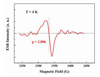
Figure 4. Low temperature ESR spectrum of the CsPbBr<sub>3</sub> QDs/mc-Si structure.
