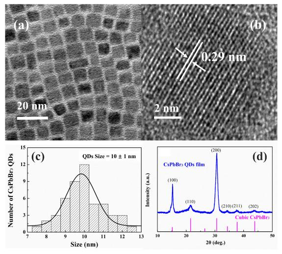
**Figure 1.** (a) TEM and (b) HRTEM images of CsPbBr<sub>3</sub> QDs. (c) Histogram for the size distribution of the CsPbBr<sub>3</sub> QDs. (d) XRD spectrum of CsPbBr<sub>3</sub> QDs film.
