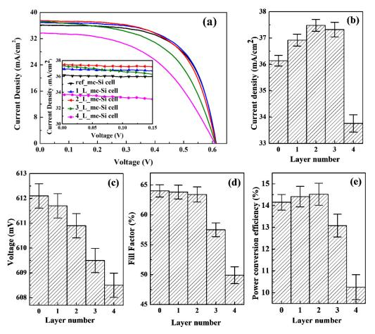
**Figure 3.** (a) AM 1.5G illuminated *J*-*V* curves of mc-Si solar cells inclusive and exclusive of CsPbBr<sub>3</sub> QDs layers. (b) Short circuit current density ( $J_{sc}$ ), (c) open circuit voltage ( $V_{oc}$ ), (d) fill factor (FF), and (e) power conversion efficiency (PCE) of solar cells.
