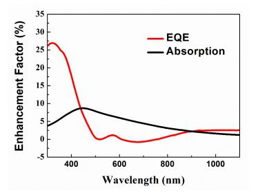
**Figure 7.** Enhancement factor (EF) of mc-Si solar cell coated with two layers of CsPbBr<sub>3</sub> QDs as a function of wavelength.
