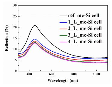
Figure 6. Optical reflection spectra of mc-Si solar cells inclusive and exclusive of CsPbBr<sub>3</sub> QDs layers.
