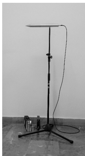
Figure 2. Measuring equipment: G.R.A.S. 67SB transducer on a tripod, bottom left, measuring the cassette of the Brüel & Kjær 3052-A-030 input module (with battery and Wi-Fi modules) and the G.R.A.S. 12AK power module.
