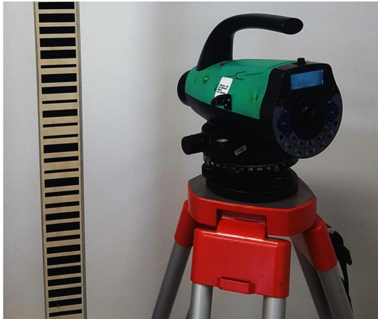
**Fig 2. Digital level—Bar-code staff system.** Example of a *digital level—bar-code staff* system [44].
