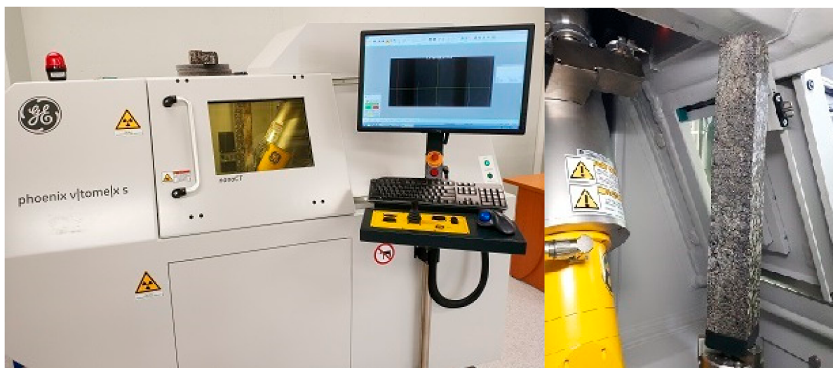
Figure 15. Computed tomography and mounted specimen.
