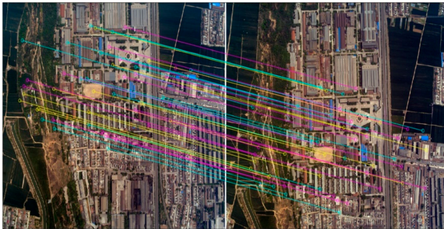
Figure 9. Partial view of the tie points obtained by SURF (showing only 50 tie points).
