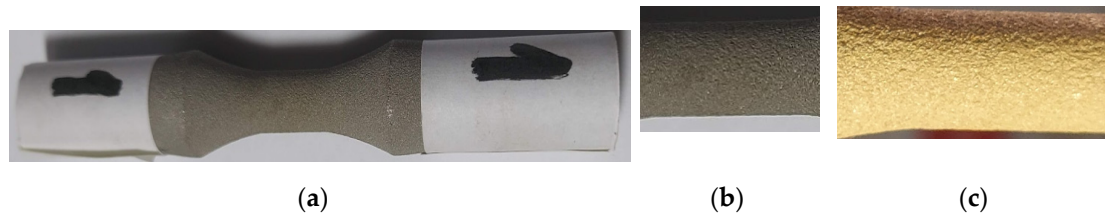
Figure 9. Macroscopic appearance of the outer surface after fatigue stress—Sample 1 \sigma_{max} = 420 MPa, N = 5,519,600 cycles. (a) the unbroken sample after more than 5 million cycles ( 8\times ). Macroscopic image of the surface for (b) 32\times and (c) 45\times magnification. Sample 8 had a similar appearance.
