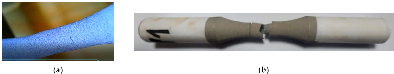
Figure 4. Sample subjected to static tensile load. (a) Image from the video that captures the moment of cracking of the coating material at the static tensile load; (b) broken sample after static tensile.
