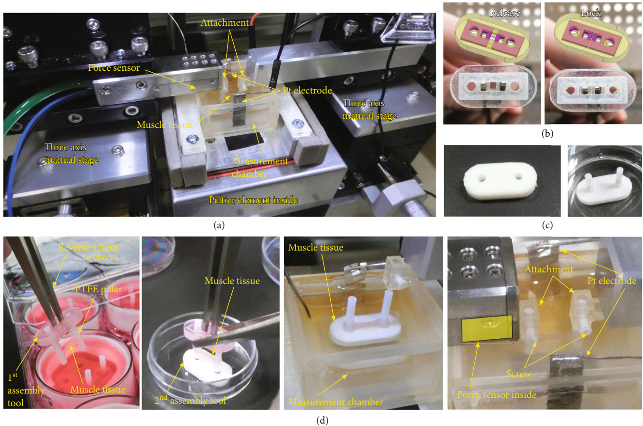
FIGURE 2: Force measurement of TEMs. (a) Photo showing the center of the force measurement system. (b) The first assembly tool. The magenta parts were not connected to the yellow part so that former parts moved freely inside the space. (c) The second assembly tool was fabricated by drilling two holes to hold the PTFE pillars. (d) Photo images for the steps to position the TEM.
