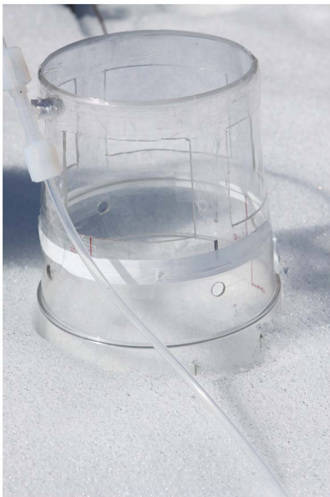
Figure 1. Modified Teflon Fluorinated Ethylene Propylene (FEP) Chamber with Polycarbonate (PC) Frame and 25 μm Teflon FEP Film Top and Side Windows. doi:10.1371/journal.pone.0069342.g001
