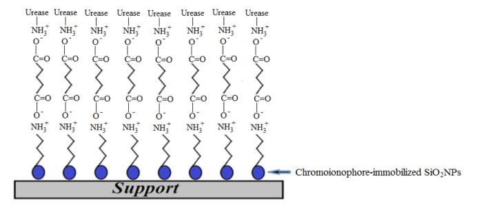
Figure 1. Schematic illustration of the SiO<sub>2</sub>NPs-based optical urea biosensor.
