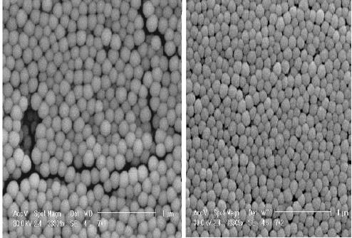
Figure 3. SEM images of  $SiO_2NPs$  for (a) t1 and (b) t2 compositions.
