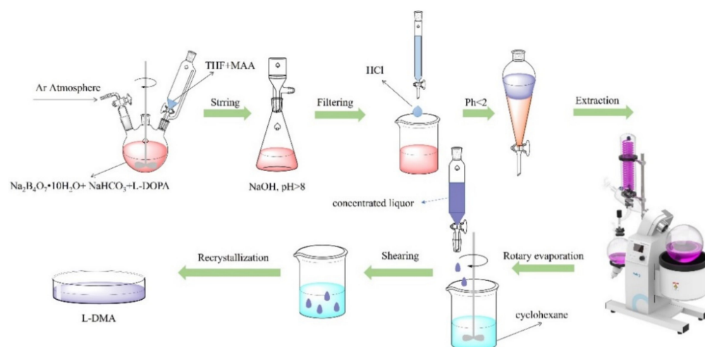
Figure 4. Preparation procedure of L-DMA.
