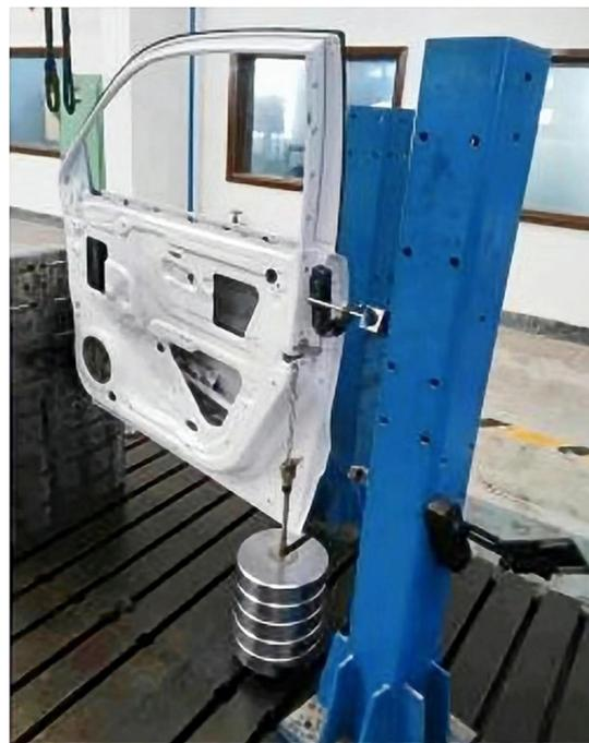
**Figure 3.** Experimental test of stiffness for the automotive door.
