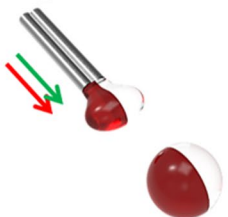
Figure 2. Generation of complex alginate microsphere. The shape of alginate microsphere is determined by changing sequences of modular micronozzle including (A) “a, b”, (B) “a ∩ b”, and (C) “a ∪ b”, respectively. The scale bars represent 3 cm.
