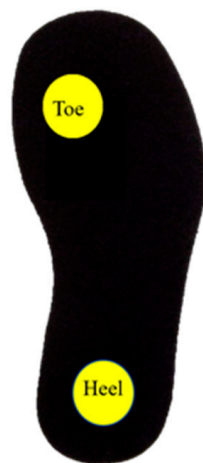
Figure 8. The position of the sensors on the heel and toe part of the insole which are related to the point with higher pressure in the sole of the foot.
