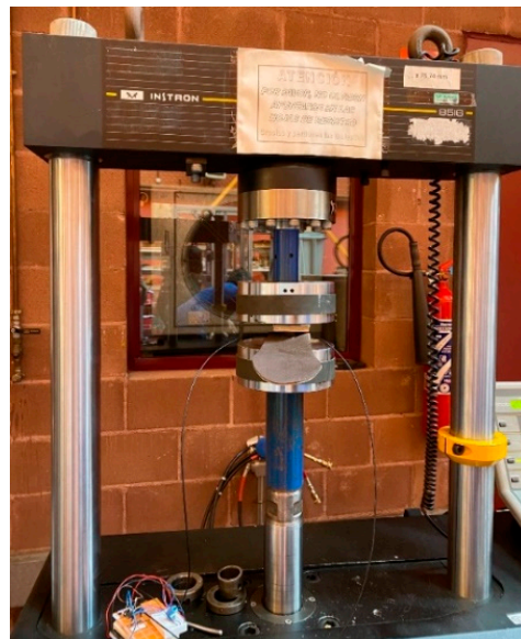
Figure 2. Photograph of the load testing platform with an EVA insole.
